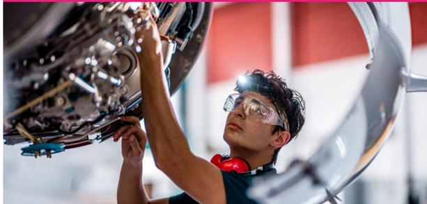
With job titles such as aircraft mechanic and aircraft fitter, people working in this role fit, service, repair and overhaul aircraft engines and assemblies.
